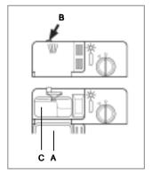
Note: To facilitate closing the cover, remove any excess detergent on the edges of the dispenser.
